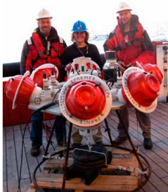
Gathering data: Dr Isabelle Ansoorge, chief scientist Marcel van den Berg, and French technician Michel Hamon about to deploy a Current Pressure Inverted Echo-Sounder (CPIES) into the South Atlantic.
